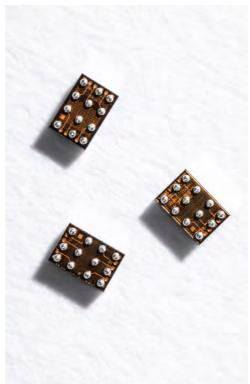
The MS8892 is available in small plastic packages like QFN16 (3x3 mm) and chip scale packages ( $1.03 \times 1.52$  mm)
