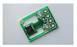
Our sensors are available in small plastic packages es like QFN16 (3  $\times$  3 mm) and chip scale packages (1.39  $\times$  0.93mm). The picture on the left shows our evaluation board with the QFN16 package.
