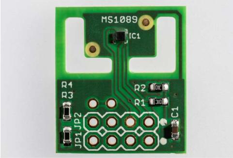
The MS1089 is a fully integrated, tested and calibrated I<sup>2</sup>C digital temperature sensor with a typical accuracy of 0.3°C from 0 to 60°C. Its temperature range is -40°C to 85°C with three selectable resolutions of 0.1°C, 0.05°C and 0.025°C, and a supply range of 1.8-3.6V.
