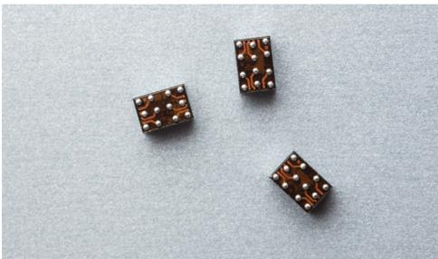
The chip scale package is supplied in tape and can be soldered like a conventional SMD component.
